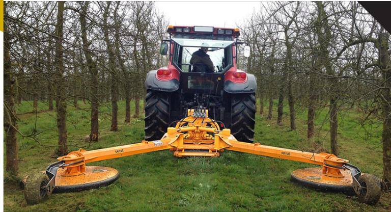
Double mechanical driven swing arms mower conceived to mow around trees, under fences, posts, crash barrier, vineyards, trees, etc. without any damage. Allowing in a single work process to clean two lines of plantation in an average speed of 3 km/h. We work with a width of 6.20/6.50 m with regard to the axis of the tractor (3.10/3.25 m in each sides).
