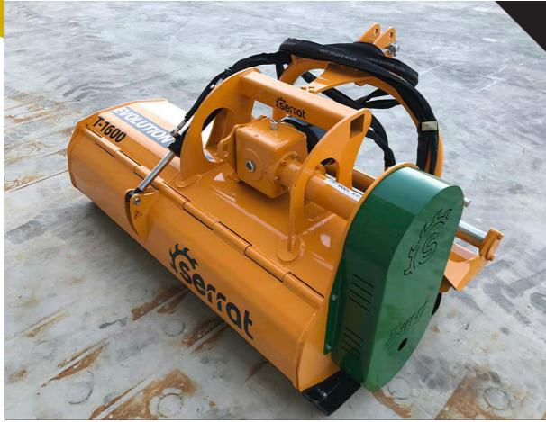
Mulcher designed for tractors between 60 HP to 120 HP for the maintenance of vegetable mantle and for the elimination of remains of pruning up to 80 mm.
